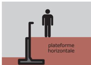
Surcharge piétonne = 5 kN/m<sup>2</sup>
